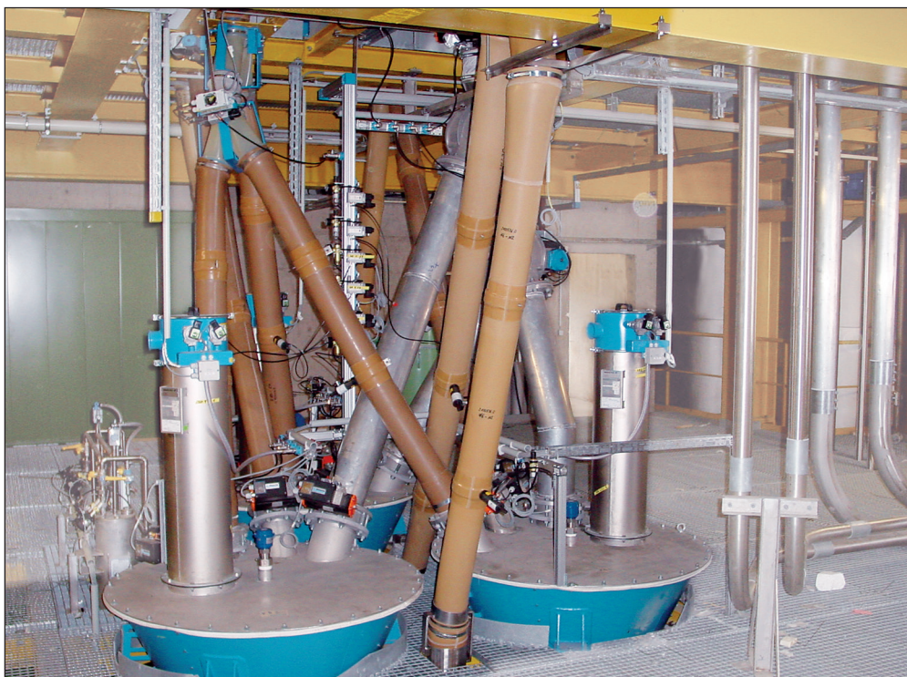
Figure: Flexible flow arrangement in a PVC mixing system
